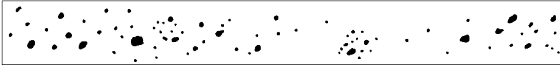
(a) Random Rounded Indications [Typical concentration and size permitted in any 6 in. (150 mm) length of weld.]
