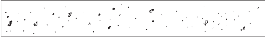
(a) Random Rounded Indications [Typical concentration and size permitted in any 6 in. (150 mm) length of weld.]
